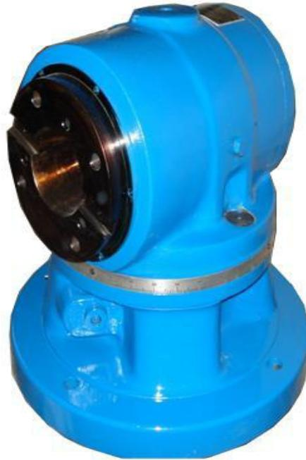
The VFW 3 Milling head finds its application mainly in milling operations performed in holes and on surfaces parallel with main spindle centerline. No resetting of Work piece is required when using the mentioned milling head.
